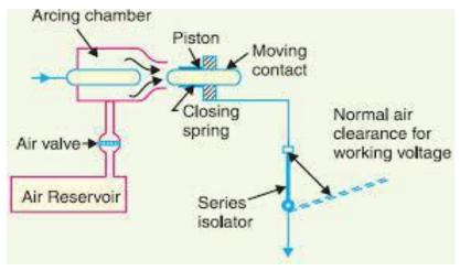
When a fault occurs the tripping impulse causes the opening of the air valve which connects the circuit breaker reservoir to the arcing chamber. The high pressure air entering the arcing chamber pushes away the moving contact against spring pressure.
