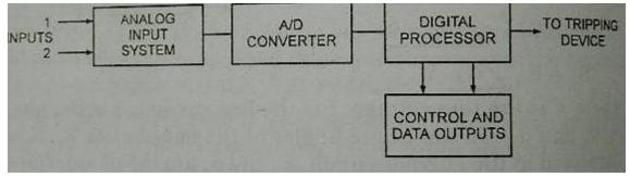
A block diagram of a microprocessor based digital programmable static relay is shown in figure.
