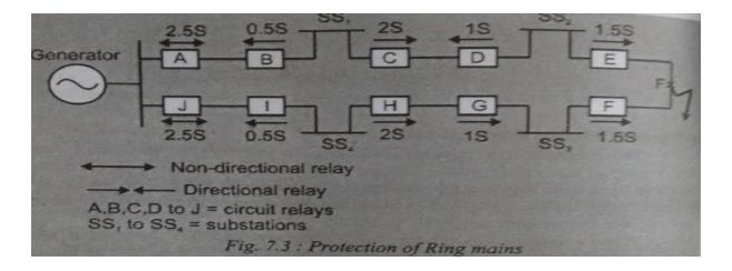
A typical ring main system consisting of one generator (G) and four substations (SS1, SS2, SS3 and SS4) is shown in fig. 7.3. Since the power can flow in both directions in this arrangement, therefore, it is necessary to grade in both directions around the ring and also to use directional relays. In order to isolate only faulty section of the ring under faulty conditions, the types of relays and their time settings should be as under.
