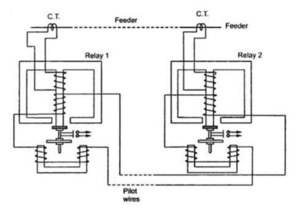
The secondaries of the two relays are connected to each other using pilot wires. The connection is such that the voltages induced in the two secondaries oppose each other. The copper coils are used to compensate the effect of pilot wire capacitance currents and unbalance between two currents transformers.
