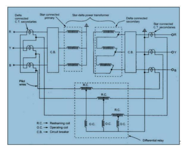
The star point of the power transformer primary as well as the star connected C.T. secondaries must be grounded. The restraining coils are connected across the C.T. secondary windings while the operating coils are connected between the tapping points on the restraining coils and the star point of C.T. secondaries.
