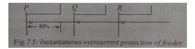
If fault in between Q and R, the relay at Q should trip. But it shout not operate for faults beyond point R. Similarly, the relays at point P should trip for fault between points P and Q. The relay at R should trip for faults beyond R. This operation is not achieved due to the following reasons.
