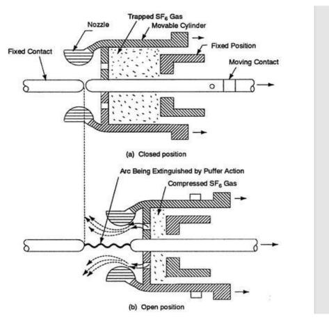
The gas pressure inside the cylinder is maintained at around 5 kgf per sq. cm. At higher pressure the dielectric strength of the gas increases. But at higher pressure the SF<sub>6</sub> gas liquify at higher temperature which is undesired. So heater is required to be arranged for automatic control of the temperature for circuit breakers where higher pressure is utilised. If the SF<sub>6</sub> gas will liquify then it loses the ability to quench the arc.
