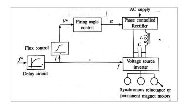
1.Sketch the block diagram of True Synchronous Mode of Synchronous Motors
