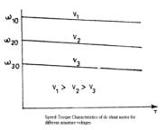
This method is only for below rated speed since the voltage magnitude should not be greater than the rated voltage. The variable voltages can be obtained by phase controlled rectifier and DC-DC Chopper
