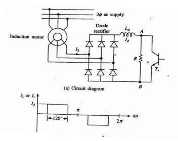
2.Draw the closed loop block diagram of rotor- resistance control using chopper (Static Rotor Resistance Control)?
