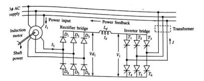
5.Draw the block diagram of Static Kramer drive with the help of a neat schematic?
