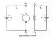
The basic equations for DC motor are  $E = K_c \phi w_m$   $V = E + I_a R_a$  $T = K_c \phi I_a$
