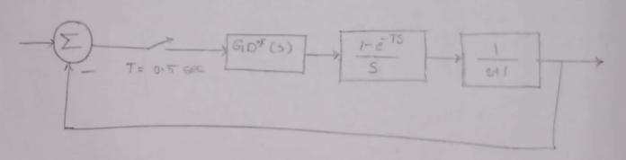
$GD^*(5) = GD(Z) = \frac{KZ}{Z-1}$  and locate the closed loop poles corresponding to K=2
