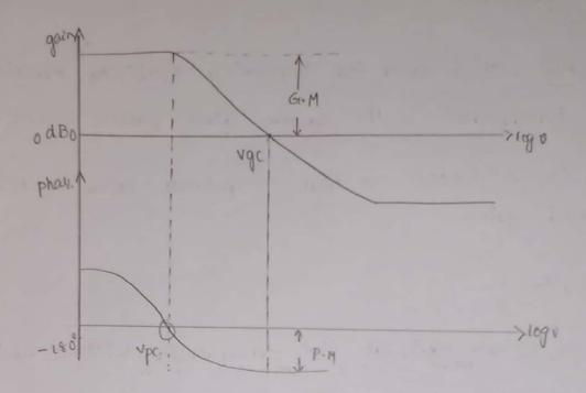
For example we have to design a compensator en order to improve gain & phan margin
