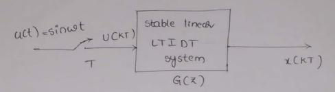
The Frequency Response of G(z) can be obtained by substituting  $z=e^{i\omega t}$  into G(z)
